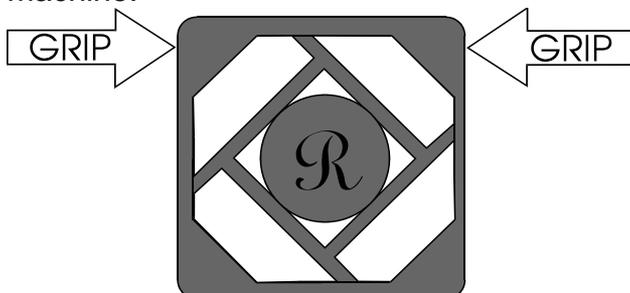
To remove the filter, grip the filter housing with the thumb and forefinger, across the top corners and pull the filter cover away from the ventilator. Remove and inspect the element. To clean the filter element, wash gently in tepid, soapy water. Rinse and allow the element to **dry**. When
