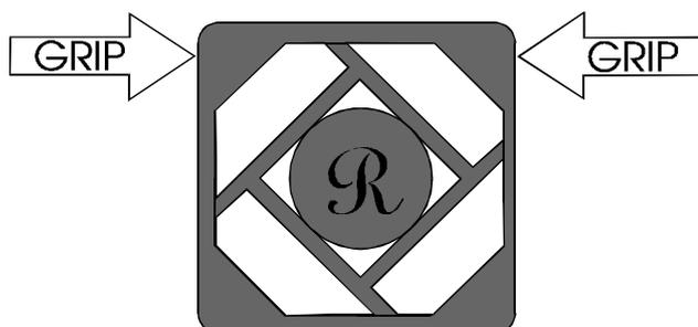
To remove the filter, grip the filter housing with the thumb and forefinger, filter cover away from the ventilator. Remove and inspect the element.
